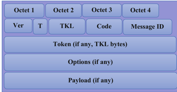
Fig. 7.6 Constrained Application Protocol (CoAP) message format
