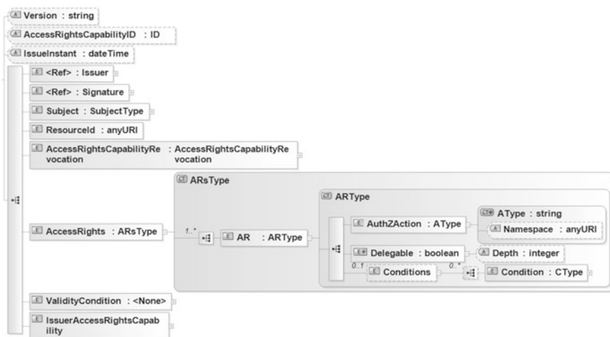
Fig. 6.6 Capability token XML schema: Access Rights Capability Type definition conveying details of the granted Access Rights (AR) type
