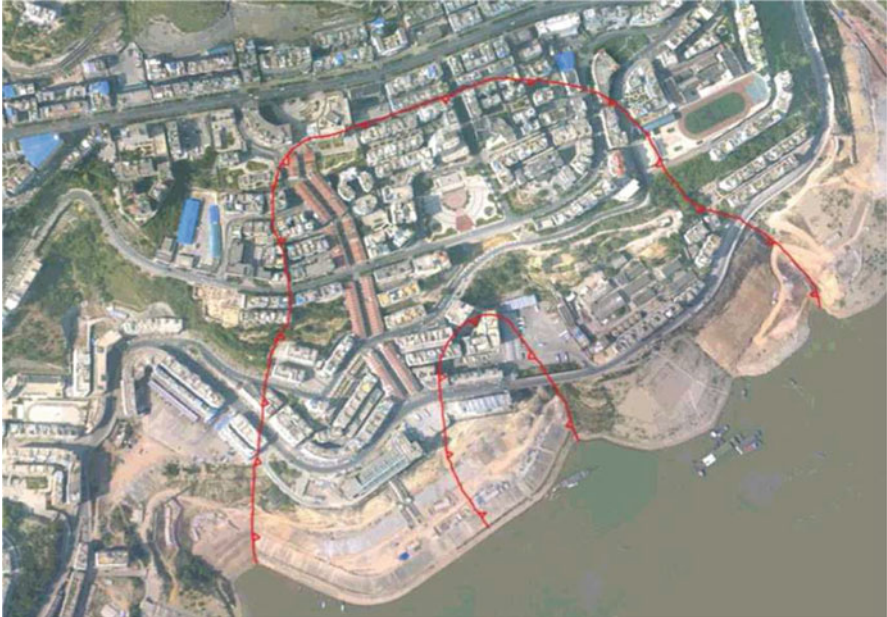
Fig. 3.2 Identify a landslide from remote sensing images
