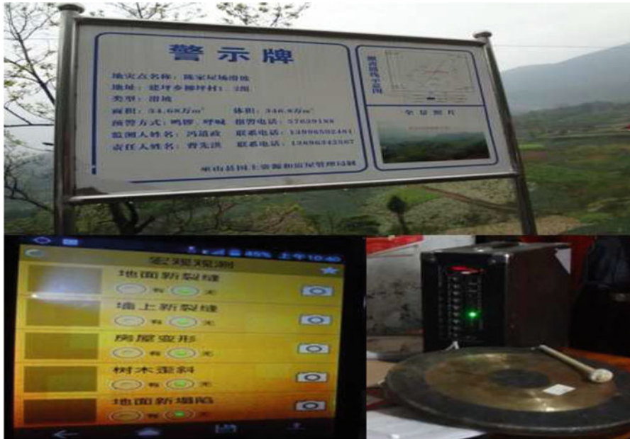
Fig. 3.7 Information bulletin of a landslide observer (the upper figures), mobile APP for reporting observations (the lower-left figure), and warning devices, a gong & a loudspeaker (the lower-right figure)
